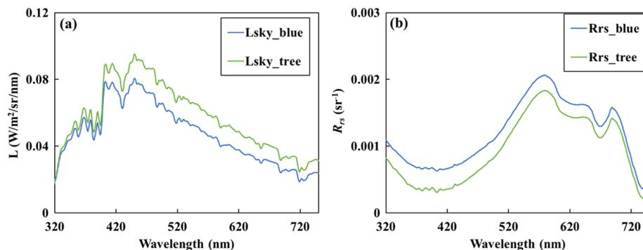
**Fig. 9.** (a)  $L_{sky}$  measured near treetops and from blue sky. (b)  $R_{rs}$  of the same location obtained from two different azimuth angles.
