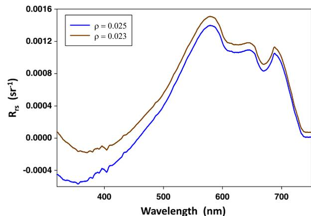
**Fig. 3.**  $R_{rs}(\lambda)$  spectrum via AWA for Station 1 of this study.
