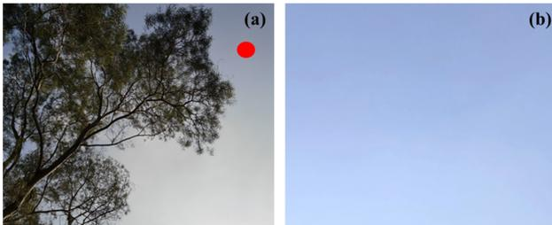
**Fig. 8.** (a) Picture of sky near treetops. The red dot represents the direction that the spectrometer was pointing for the measurement of  $L_{sky}$ . (b) Picture of blue sky.
