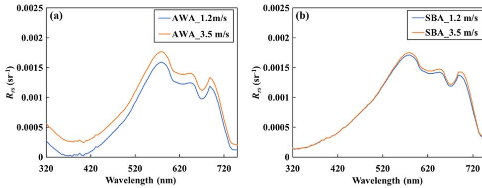
**Fig. 7.**  $R_{rs}$  spectra obtained under different wind speed at Station 3: (a) obtained  $R_{rs}$  via AWA and (b) obtained  $R_{rs}$  via SBA.
