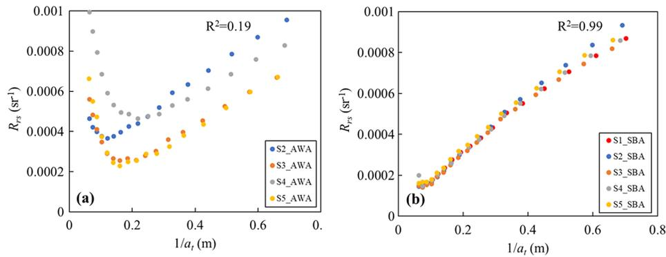
Fig. 5. Scatterplots between  $1/a_t$  and  $R_{rs}$  for wavelengths in the range of 320–480 nm (every 10 nm): (a) for  $R_{rs}$  measured by AWA and (b) for  $R_{rs}$  measured by SBA.
