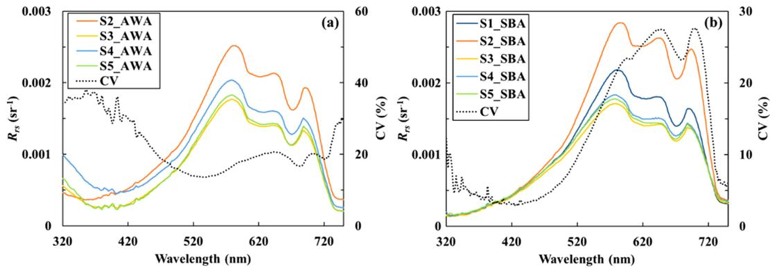
**Fig. 2.** Spectra of  $R_{rs}(\lambda)$  along with their coefficient of variation (CV) of this study: (a) obtained via AWA and (b) obtained via SBA.
